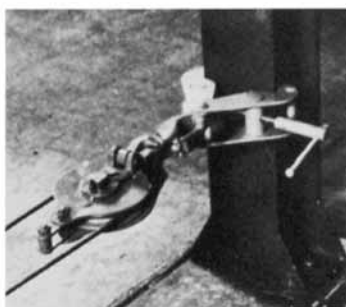
Rigging Anchor Point
